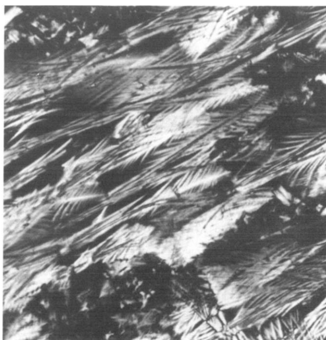
Figure 2 Dendritic-shape TCX crystallites precipitated out of a 30 phr GPPS/TCX system. Cooling rate, 10° C/min (Mag. 150X)
